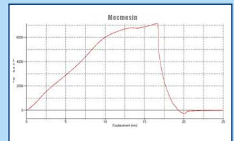
Rigidity testing of carrageenan gel
