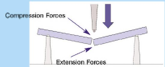
Significant stress is created within the sample to the point where failure occurs and the sample breaks.
