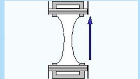
Sample is fixed at base. Top jaw moves up and sample is extended until a break is caused at the weakest point.
