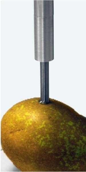
Cylinder probes may be used to perform puncture and penetration tests on a wide variety of food products including baked goods, confectionery, dairy products, fruits and vegetables and meats. Precision engineered stainless steel, perspex or acetate probes are included in our standard range. Custom designs and geometries are available on request.
