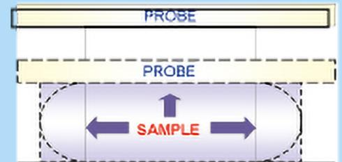
Geometry of samples changes as it is squashed. Friction is generated at test interface. The probe area, by definition, should remain greater than the sample surface area.
