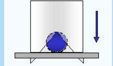
Sample is located beneath the shear blade. Stress increases as blade moves down until sample yields and blade starts to cut through.
