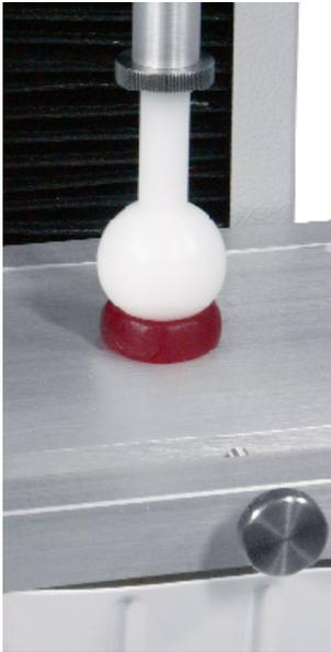
For determining surface hardness of products such as cheeses, fruits and vegetables, or the fracturability of potato chips, the spherical probe range features precision-engineered stainless steel ball-end probes, and plastic hemispherical probes which replicate squeezing in hand.
