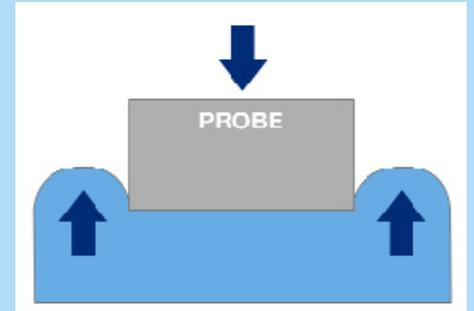
Probe has surface area smaller than that of sample. Probe will puncture sample when sufficient stress is reached, resulting in irreversible damage to the sample.
